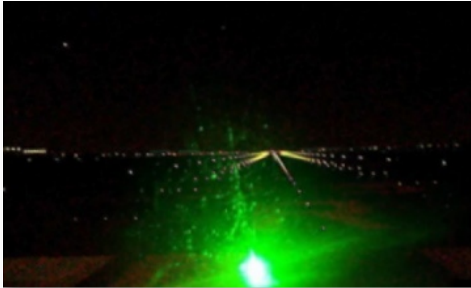
Figure 1, Distraction: FAA flight simulator showing that the light does not obscure runway lights in the background, but it is bright enough to distract the pilot. Irradiance in this photo is 0.5 \mu\text{W}/\text{cm}^2 ; for example, a legal 5 mW laser pointer at 3,700 feet (1,130 m).
